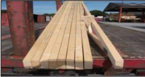
8. Once this wedge is in place the driver will then strap if possible, the remaining bundle to the centre bars leaving the separated truss to be off loaded.
