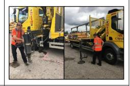
4. Wearing of the remote controller is important, the strap needs to be around the neck and over the shoulder and not just around the neck. When just around the neck if you bend the controller will swing away from the body and if not deactivated there is
