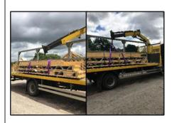
**7.** Lift slowly to ensure the load is balanced, if not lower down and adjust the slings. Ensure no persons are within the lift area
